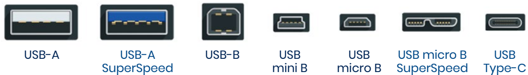
Figure 4 Predominant USB connector types (male plug shown, not to scale)
